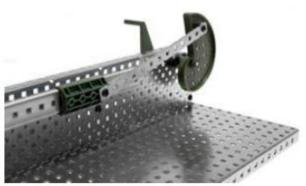
Crank and Slider - A pivot pin near the outside edge of a wheel or disk that changes \_\_\_\_\_ motion into \_\_\_\_\_ motion.
